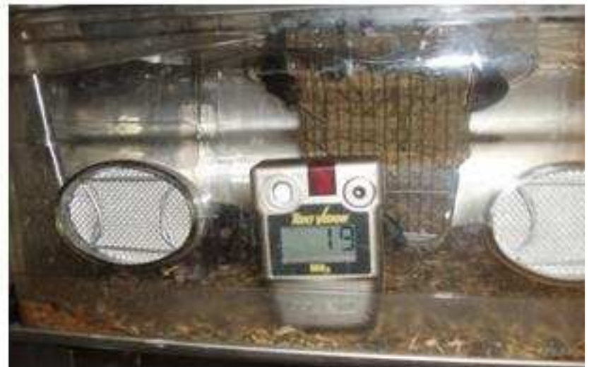
Cage Conditions: 22 °C, 67% RH, 19 ppm NH 3 15 weanies (6 weeks old); Bedding change 20 days ago
